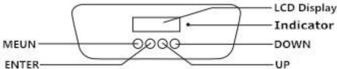
To view or modify the function settings of the lamp, press any key (in the power-on state) to light up the screen, and then press the UP and DOWN keys
